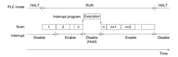
Note) The held interrupt requests are accepted when interrupt status is changed to enable, according to the priority as follows.
